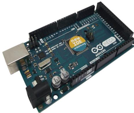
Figure 1. Arduino Mega 2560
