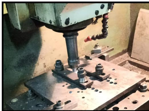
Fig.1. Welding setup used in this study
