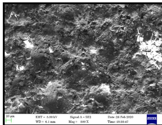
Fig.3 SEM micrograph of base metal
