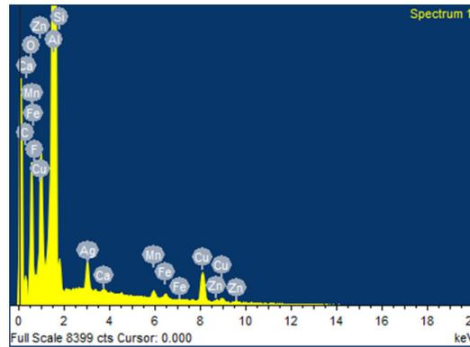
Fig.7 EDS spectrum of weld zone
