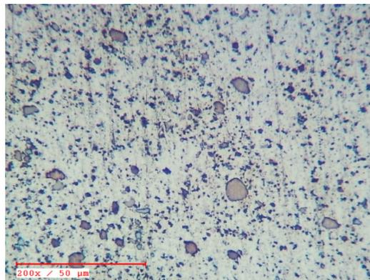
Fig.4 Optical micrograph of Weld zone
