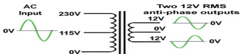
Basic power supply is the input power transformer has its primary winding connected to the main (line) supply. A secondary winding, electro-magnetically coupled but electrically isolated from the primary is used to extract an AC voltage of suitable amplitude, and after further processing by the PSU, to drive the electronics circuit it is to supply.
