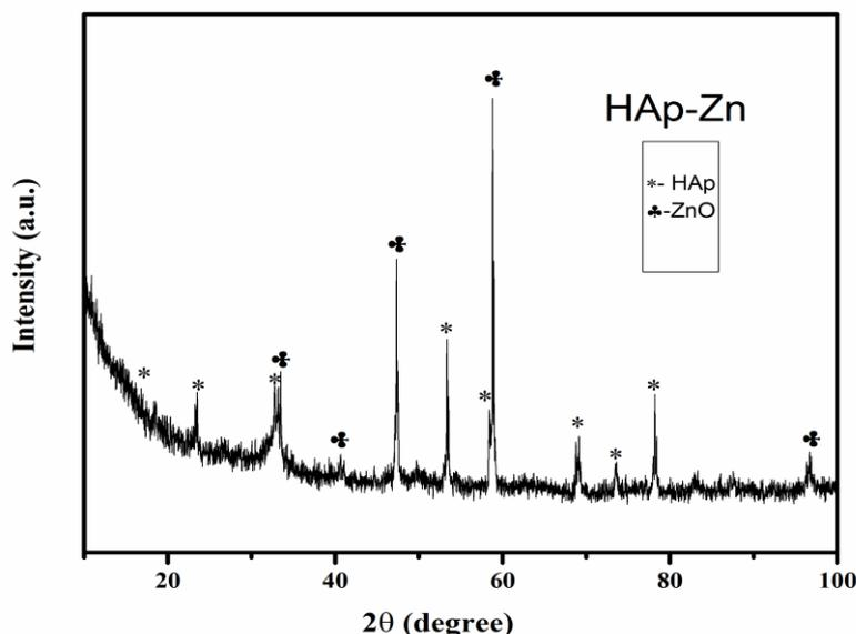
Fig.(1) XRD pattern ZnO doped HAp sample
