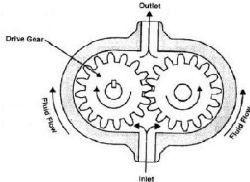
**Fig. 1.1 External Gear pump**
