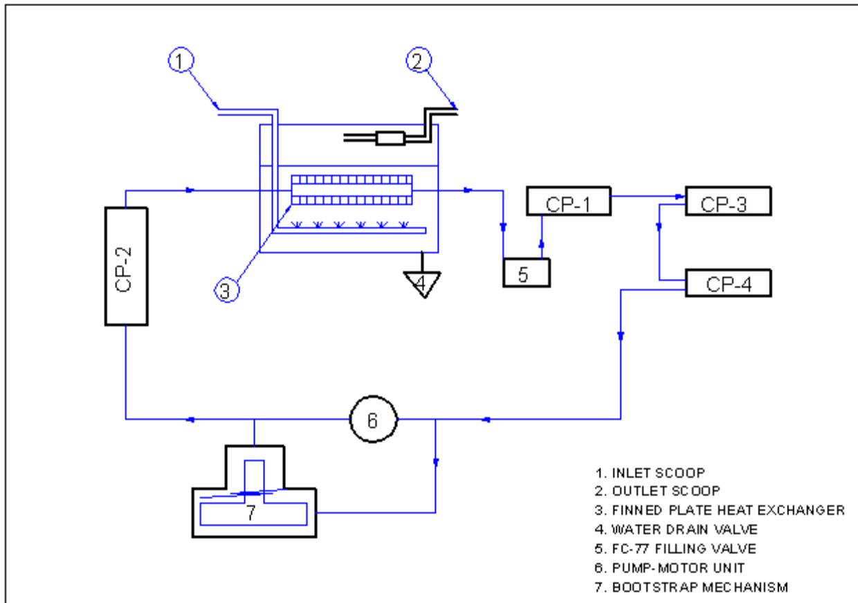
Fig-3.1 Schematic Diagram of Cooling System
