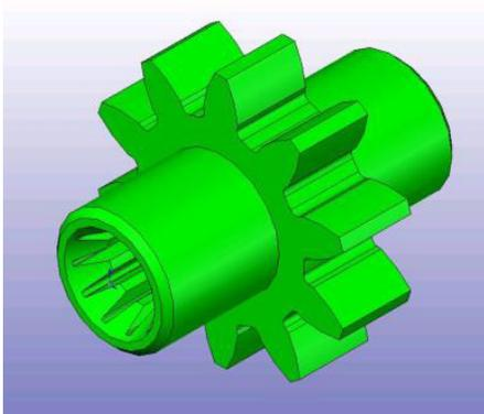
Fig. 2.2 Driver gear shaft
