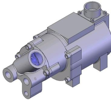
Fig. 2.1 Pump motor unit assembly
