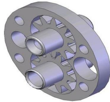
Fig. 2.3 Drive and Driven gear shaft assembly
