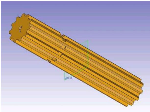
Fig. 2.13 Spline shaft
