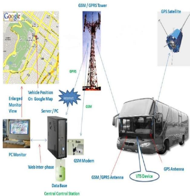
Figure 1.1: Architecture of Real Time Vehicle Tracking System
