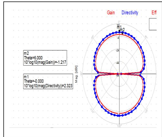
Figure 7: Gain and Directivity of the Antenna
