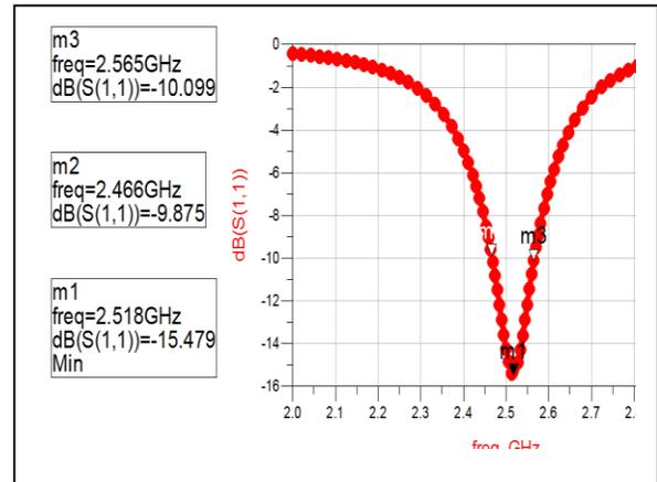
Figure 6: Simulation Result of Antenna
