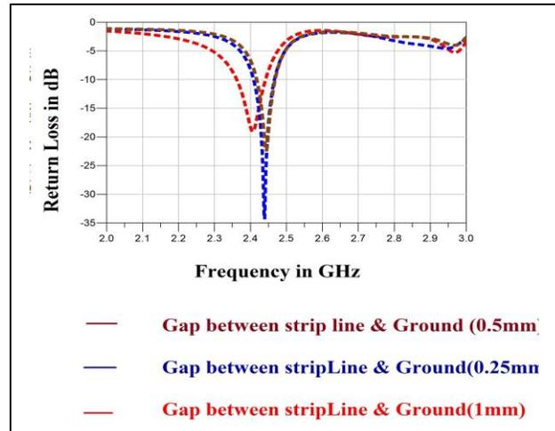
**Figure 2: Effect of gap between strip and ground**
