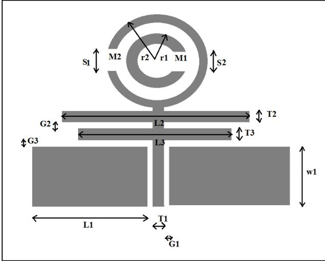
**Figure 1: Proposed Antenna Structure.**
