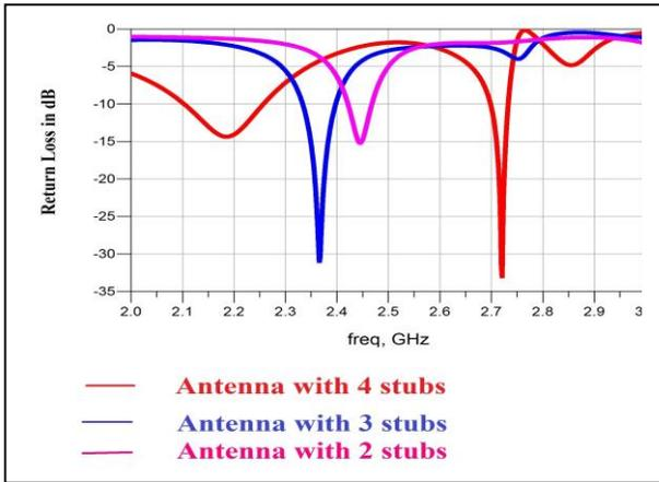
Figure 3: Changes while using different number of stubs
