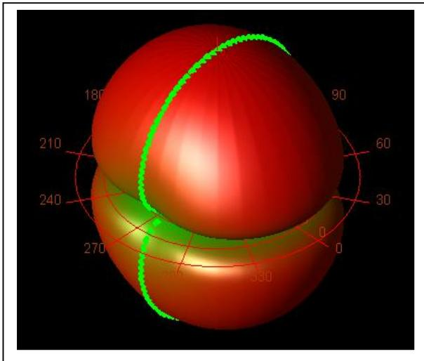
Figure 8: 3-D Radiation Pattern
