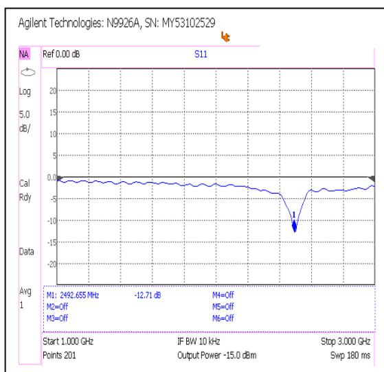
Figure 10: Return loss (dB) Measurement.
