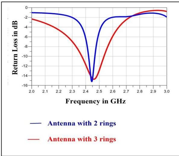
Figure 4: Comparison between Antennas with different number of rings
