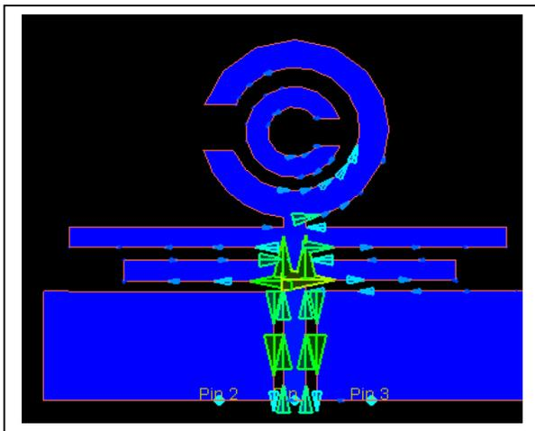
Figure 5: Current Distribution of Rectangular Ground Structure
