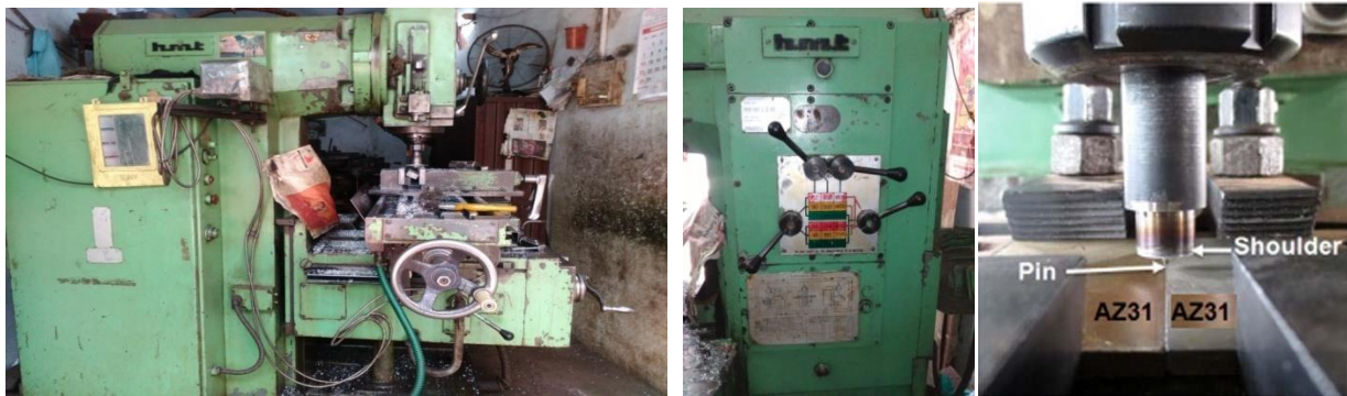
Fig-2: FSW on vertical milling machine.
