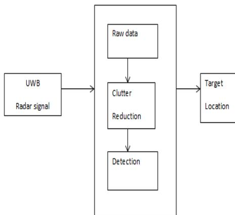
Fig 1.1 Detection of The Target With The Clutter Removal
