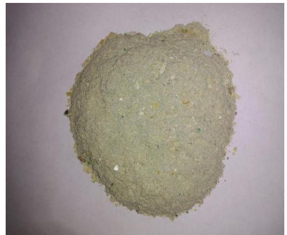
Figure 1: Powdered waste printed circuit board
