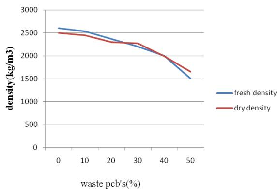
Figure 3: Density vs PCB %
