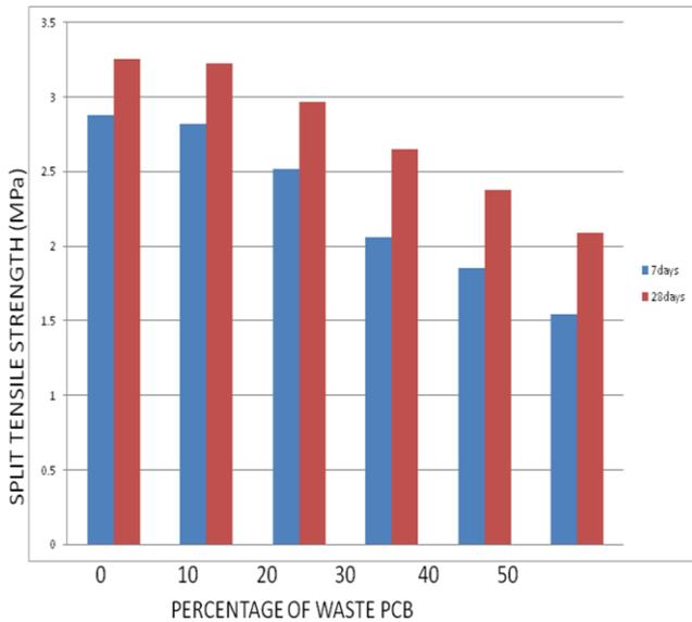
Figure 7: Split tensile strength VS PCB content.
