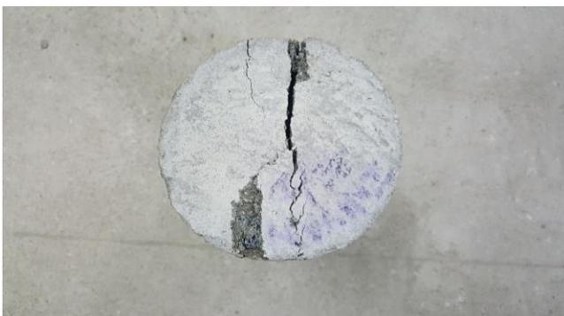
Figure 8 : Failure mode of concrete specimen
