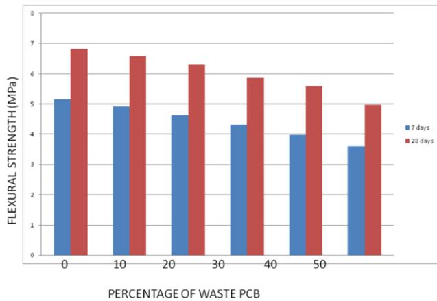
Figure 10 : Flexural strength VS PCB content.
