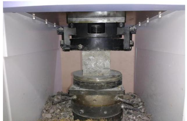
Figure 4:Specimen under compression
