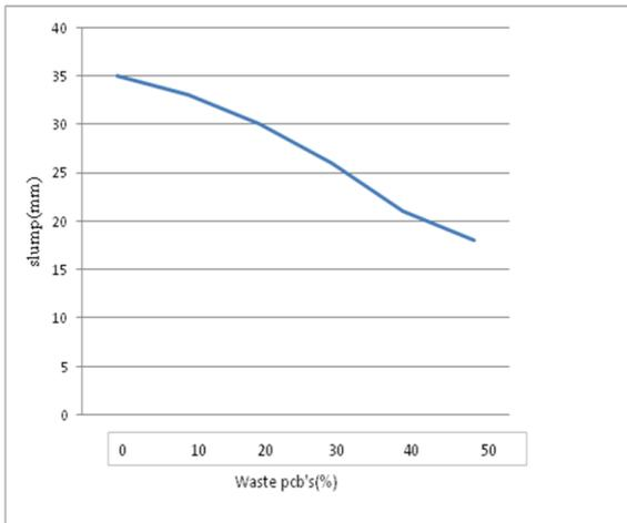
Figure 2:Slump vs PCB %
