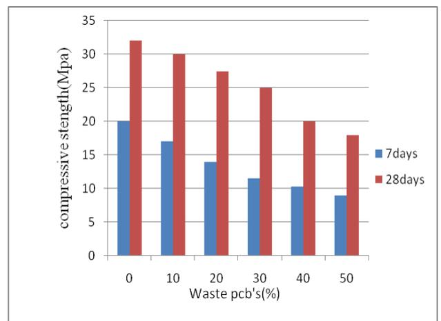
Figure 6:compression strength VS PCB%
