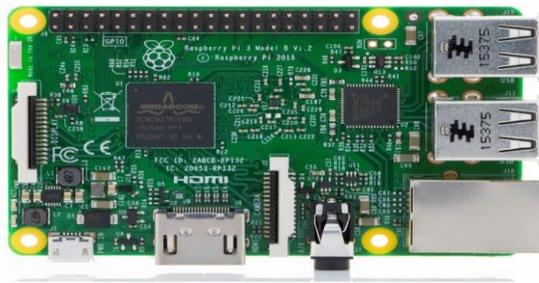
Fig1: raspberry pi 3 model B version 2
