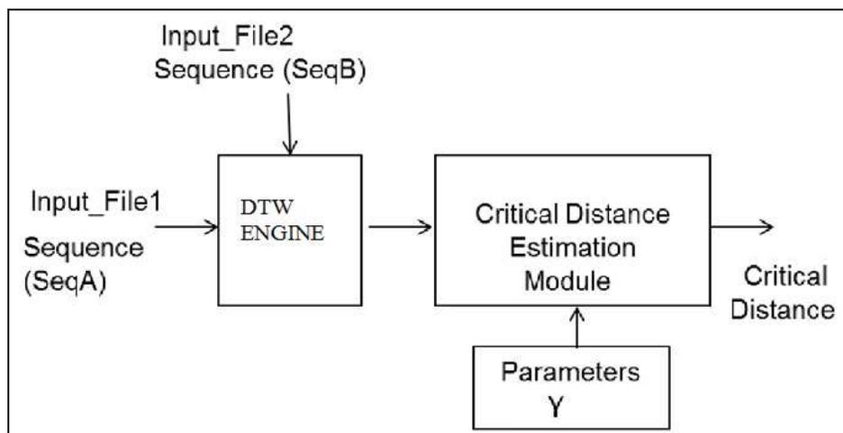
Figure 4.1: Experimental setup for estimation of critical distance
