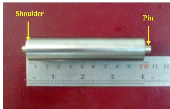
Figure 1. Photograph of FSW tool used
