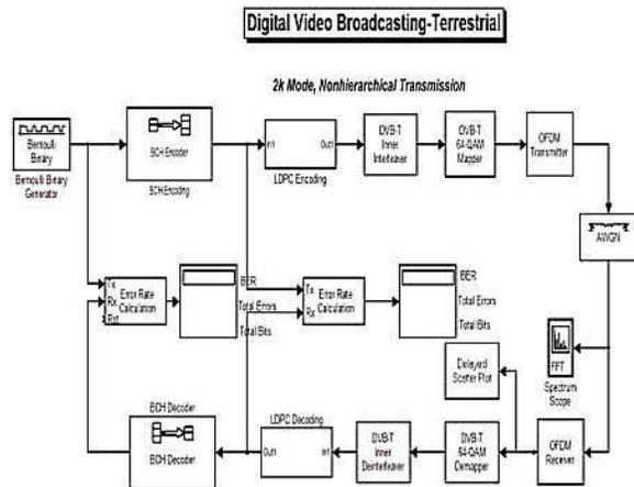
**Fig 1.** Simulink design of DVB –T2 using BCH and LDPC codes.
