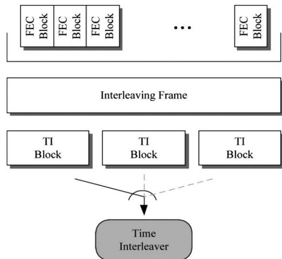
**Fig.2. Time interleaving in DVB-T2. In the figure, one interleaving frame is partitioned into three TI blocks.**
