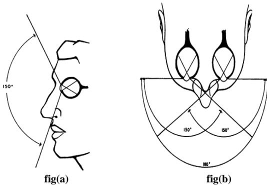
**Figure 2.2.1.1.** Human field of view: (a) vertical, (b) horizontal
