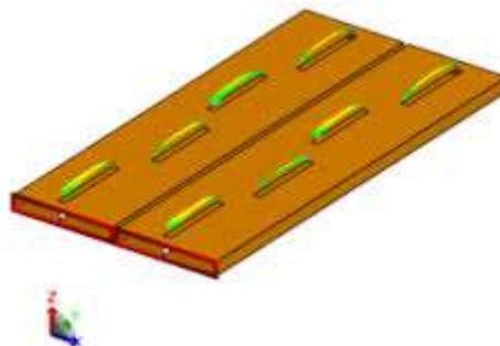
**Fig. 1: Slotted Rectangular waveguide**
