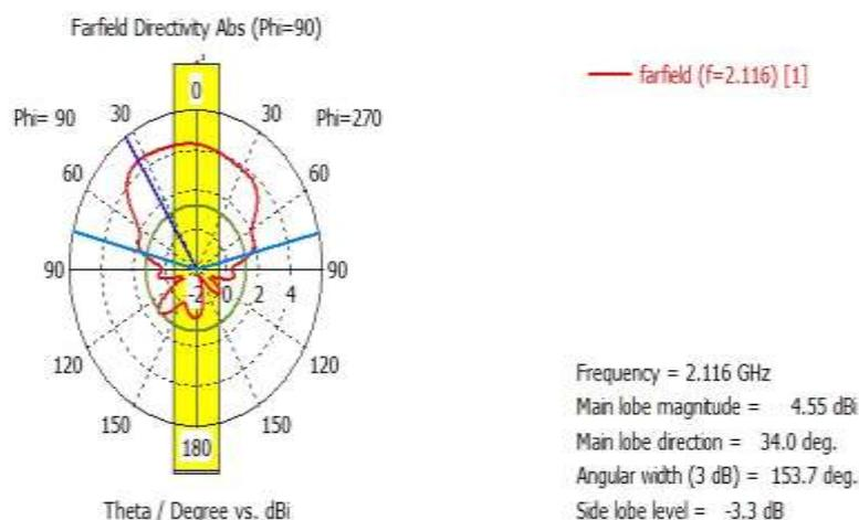
**Fig.5:Radiation pattern of a Rectangular Slotted Waveguide Antenna**
