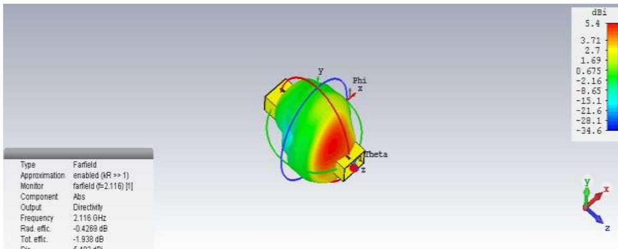
**Fig.4:Directivity of a Rectangular Slotted Waveguide Antenna**
