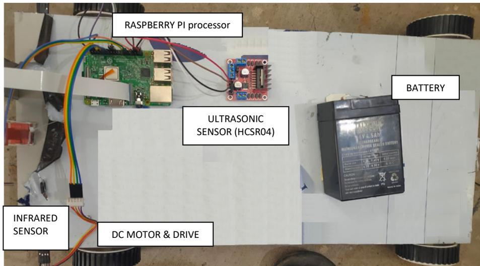
Figure.4 Model of defect detection system.
