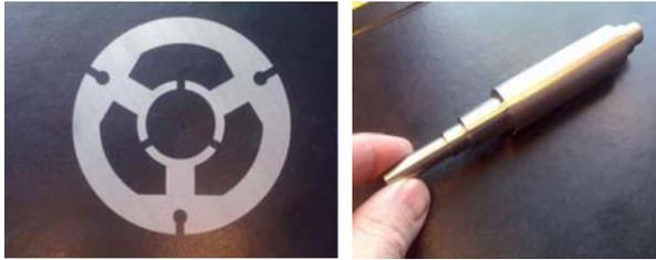
Fig. 3. Single stator lamination sheet on the left and the assembled PM rotor on the right. The magnetic circuit form is designed to reserve rectangular spaces for the cross-sections of the aramid-strip-insulated conductors.
