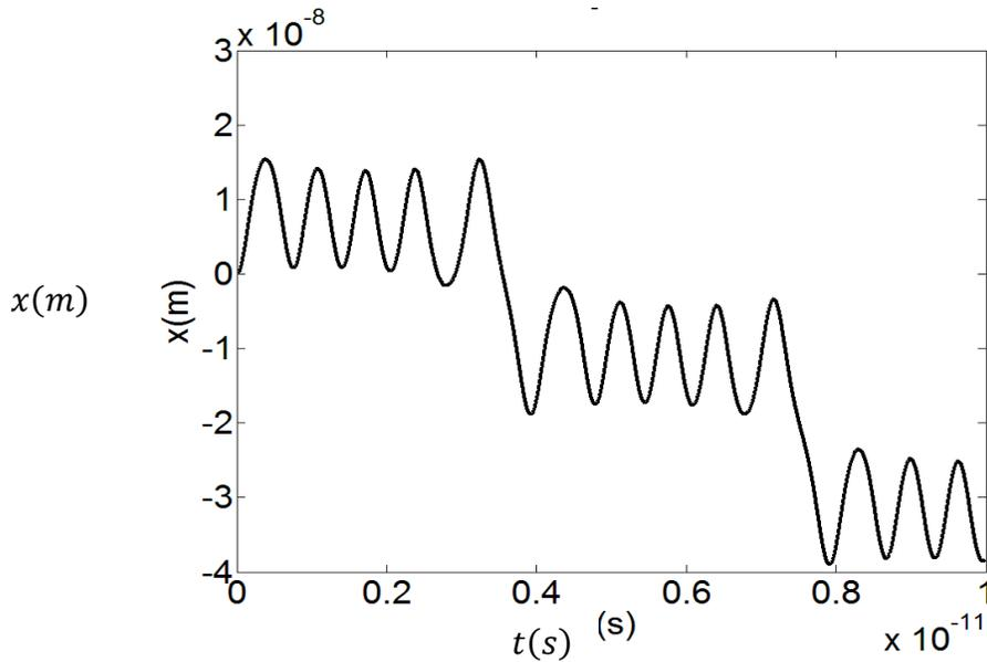
Figure 3.0: Electron trajectory when the wave amplitude,  $U = 7\text{meV}$ . The frequency oscillations are interrupted by jumps in the negative  $x$  – **direction**.
