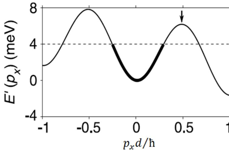
Figure 2.0: The modified dispersion relation is plotted against the momentum showing electron transport in the potential well. The wave amplitude must be greater than the miniband for the electron to traverse over the barrier. At the arrowed peak  $E'(p_x) = U_c$  refer to as the critical value. The figure is adapted from reference [3].
