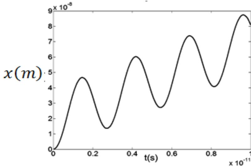
Figure 1.0: The electron trajectory in real space when the wave amplitude,  $U = 1\text{meV}$ , initially at  $x = 0$  and  $p = 0$ , the electron is being dragged in the SL with the velocity of the acoustic wave.
