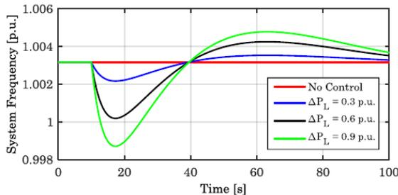
**Fig. 5. Rotor speed response during system frequency disturbance. Inertia controller gain adjusted at  $H_{syn} = 28.0$  sec.**
