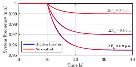
**Fig. 3. System frequency dynamic response during system frequency disturbance considering three different power imbalances**
