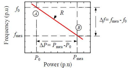
**Fig. 1. Frequency droop characteristic.**
