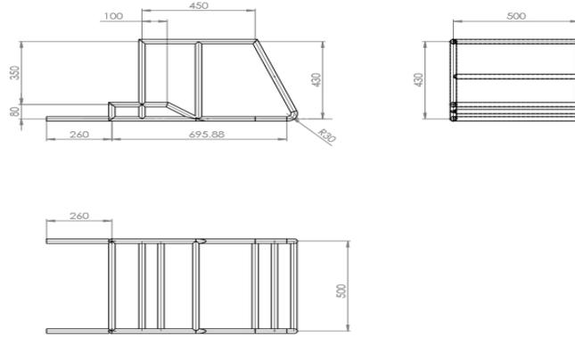
**Fig.1 Orthographic view of frame**
