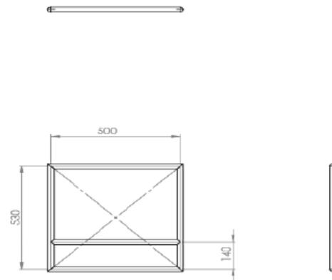
**Fig.2 Orthographic view of back rest**
