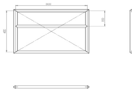
**Fig.3 Orthographic view of leg rest**
