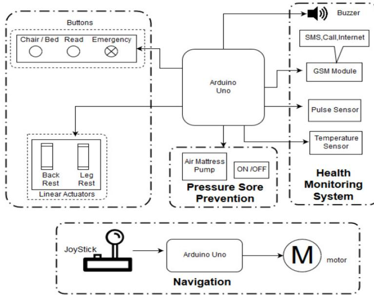
**Fig.6 Electrical circuit for automatic multipurpose bed cum wheel chair**
