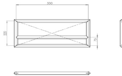
**Fig.4 Orthographic view of foot rest**
