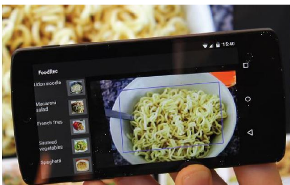
Fig. 3 Screenshot of the proposed mobile application for the food recognition problem. The bar on the left shows the first 5 classes recognized by the system for the current frame.
