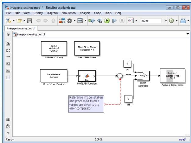
Fig 5. showing the modeled system for processing and controlling
