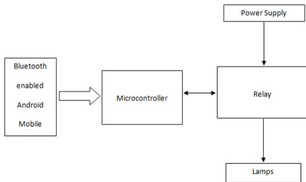
Fig 3. Block diagram showing Wireless Control
