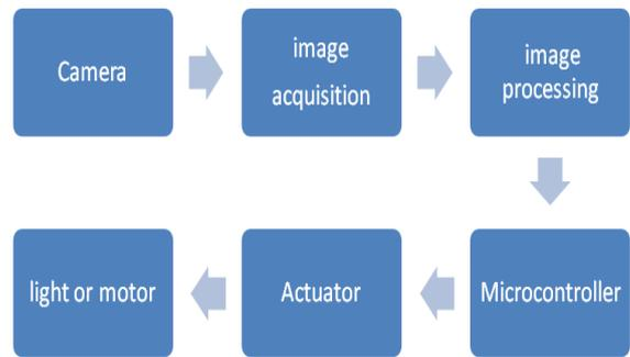
Fig 4. Block diagram showing the steps involve in automating the lighting systems
