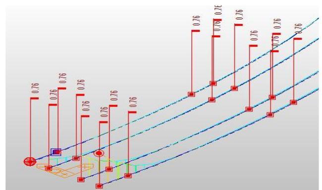
Fig 11: Position of Live load for Moving load analysis.
