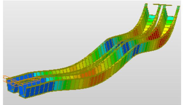
Fig 10: Displacement contour of box type curved girder during Construction stage 1
