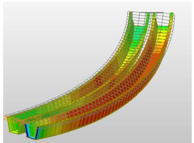
Fig 16: Bending stress contour in Box girder model
