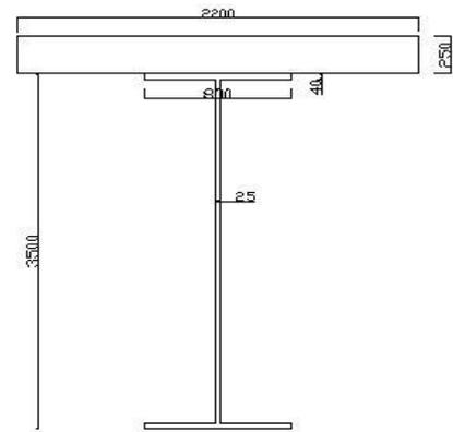
Fig 1: General section for I Girder Curved Bridge
