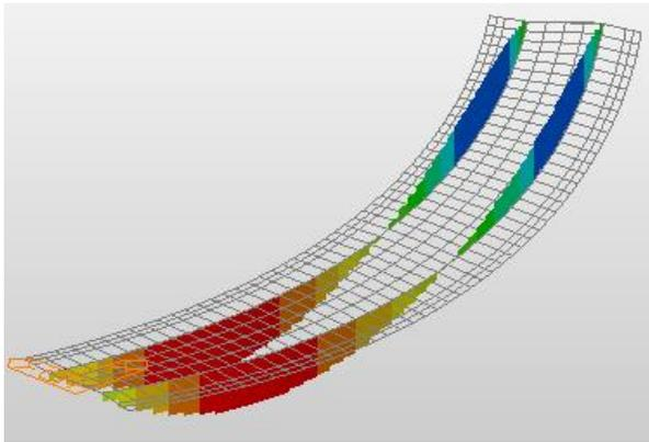
Fig 13: Torsional moment diagrams in Box girder bridge model
