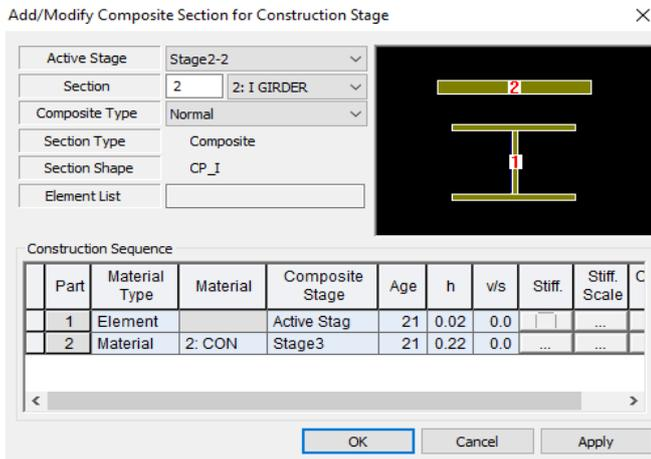
Fig 8: Activation of Composite section during Construction stage
