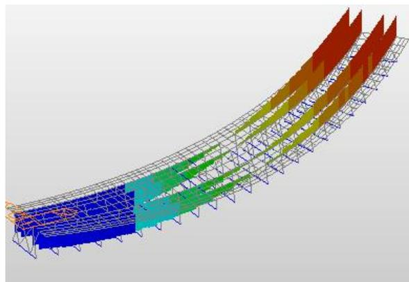
Fig 14: Torsional moment diagrams in I girder bridge model
