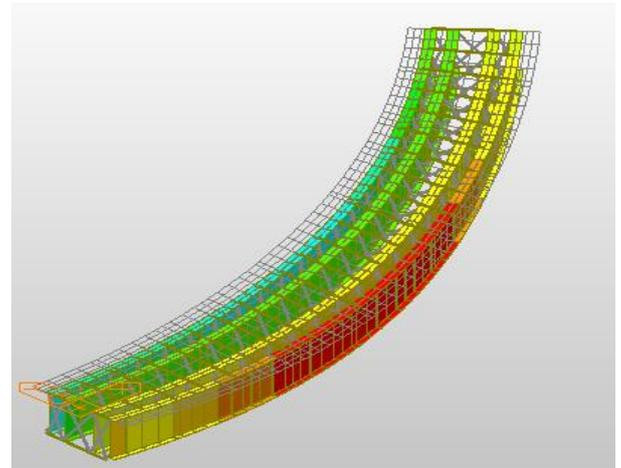
Fig 15: Axial Beam stress contour in I girder model
