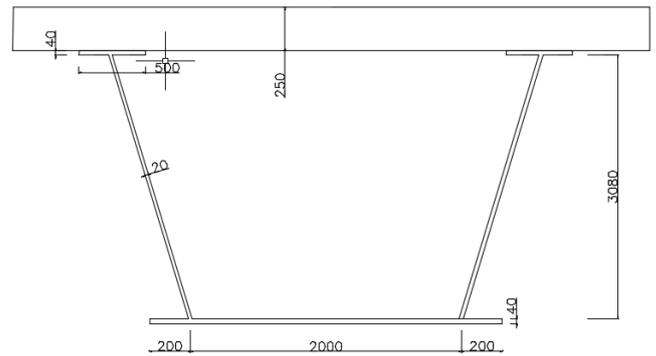
Fig 2: General section for Tub Girder Curved Bridge
