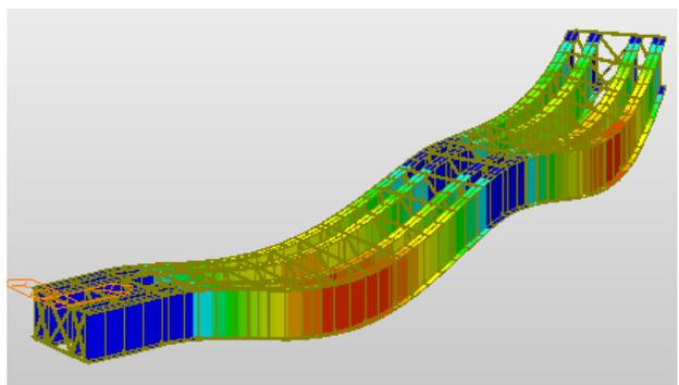
Fig 12: Displacement contour of I type curved girder during Construction stage 1
