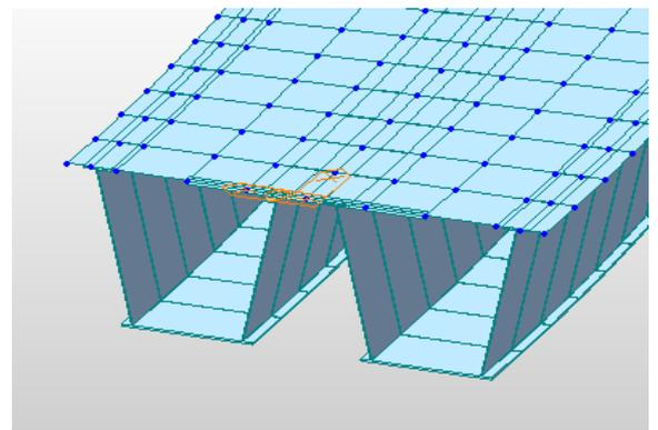
Fig 3: 3D Model of Curved Tub Girder
