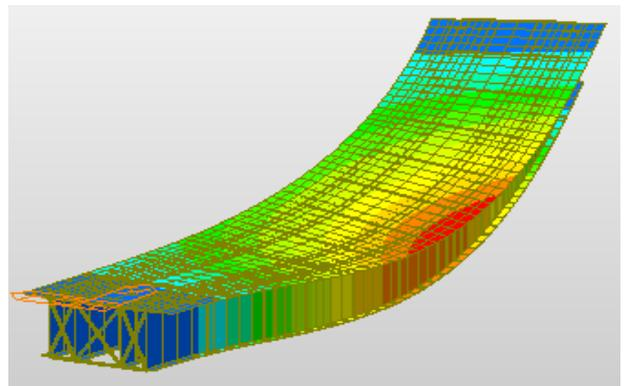
Fig 11: Displacement contour of I type curved girder
