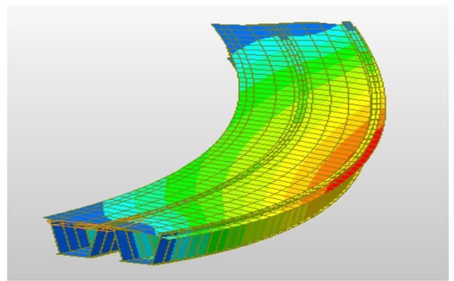
Fig 9: Displacement contour of box type curved girder
