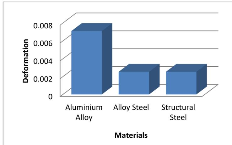
**Figure 8: Comparison graph of the Displacement**
