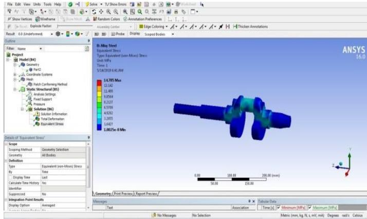
Figure 3: Total stress produced in Alloy Steel material
