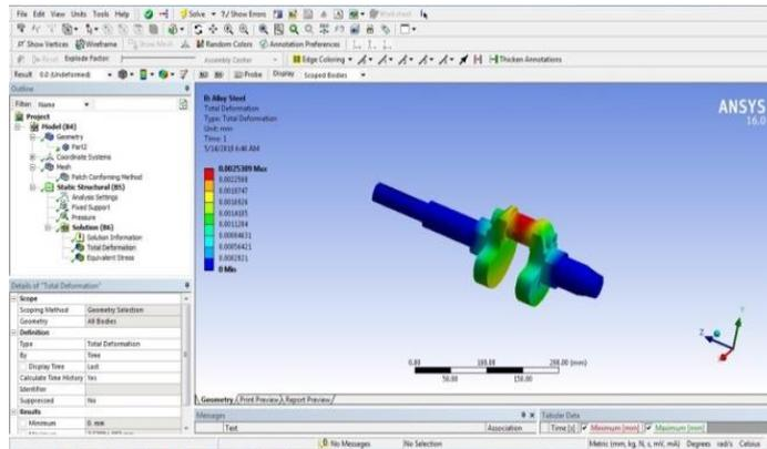
Figure 4: Total deformation produced in Alloy Steel material
