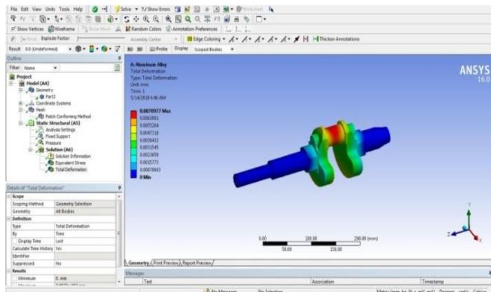
**Figure 2: Total deformation produced in Aluminium Alloy material**
