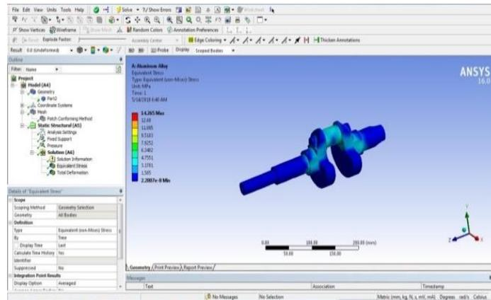
**Figure 1: Total stress produced in Aluminium Alloy material**
